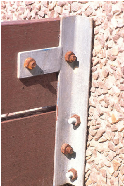
Figure 1: An assortment of zinc coated bolts showing the importance of coating thickness in a particular environment.
