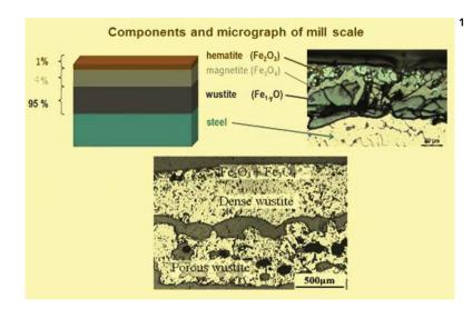
The Hematite phase,  $Fe_2O_3$  is the outer most layer of the scale and has the highest oxygen content. Hematite occupies around 1% of the total scale layer at high temperatures. As with the Magnetite phase, Hematite is hard and abrasive.
