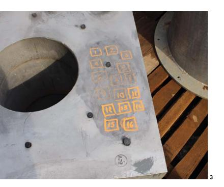
3 Reference areas: The above mentioned patched area covered roughly 16 times the refurbishment area allowed of 10cm<sup>2</sup> and <0.5% of surface area of the article hot dip galvanized [SANS121:20011 (ISO1461:2009(E))] However readings showed that the coating thickness once the patch material had been removed, was well in excess of the required coating thickness specified in the standard.
