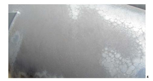
• The design of the article, in particular any concentration of a mass of steel that retains heat.
