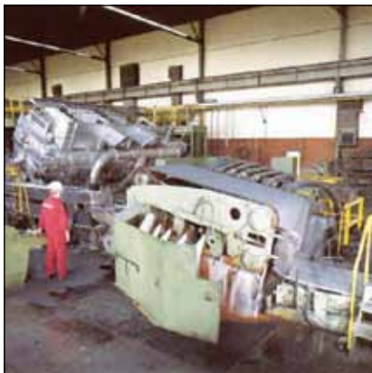
Figure 13: In the casting machine the finished alloy is provided with the input cross-section necessary for the rolling process with simultaneous cooling.
