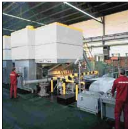
Figure 14: At the end of the rolling train the finished strip is wound into large coils and stored temporarily for cooling.
