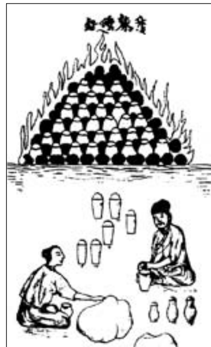
Figure 2: Production of zinc in 17th century China, using crucibles stacked into pyramids with charcoal between the spaces. After being heated until it was red-hot and subsequent cooling, the slag was broken apart to find the zinc in the middle (according to Habashi).
