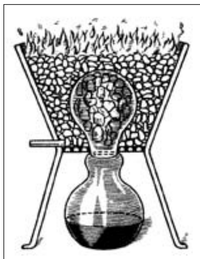
Figure 1: In India around 1200 AD metallic zinc was produced in a covered crucible. From there it passed into a condensation recipient, where it was cooled by the ambient air (according to Habashi).
