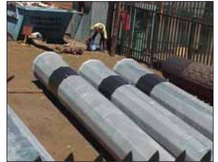
A paint film extending some 200 – 300mm above and below the ground level will prevent differential aeration.
