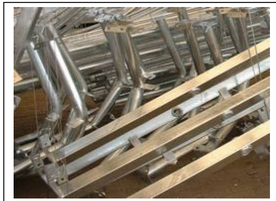
Coating thickness range between 50 to 70µm and surface finishes have a bright silvery shine. Given time (3 to 4 months exposure) all surfaces form a uniform dull grey patina of ZnCO_3 , refer to Information Sheet No. 11 “How does zinc protect?”
