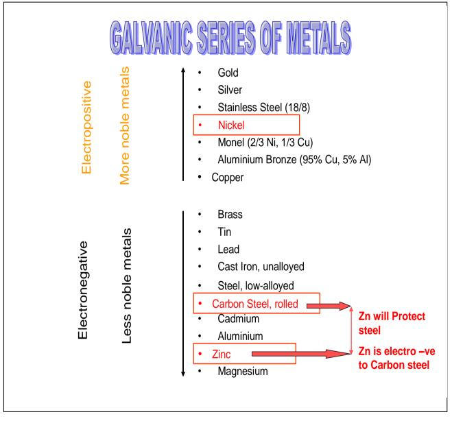
Figure 3: An example of the Galvanic Series of metals immersed in sea water. Refer to Information Sheet No.11 "How Does Zinc Protect"
