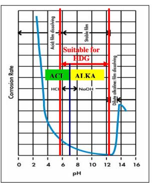
Figure 2: The reaction of pure zinc in a varying pH environment
