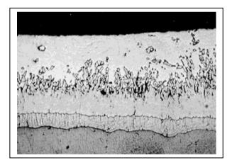
Typical micrograph of a hot dip galvanized coating using "aluminium killed" carbon steel (Silicon < 0.03% and zinc temperature 450°C)
