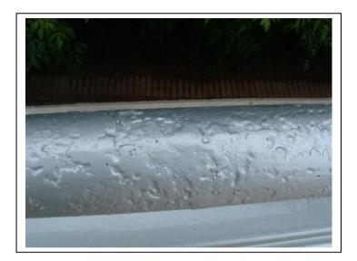
Surface appearance of reactive "silicon killed" steel with a phosphorous content > 0.02%
