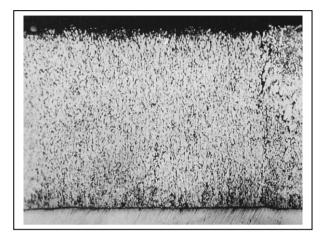
Cross-section through zinc coating on siliconkilled steel with 0.06% Si
