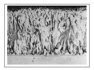
Coating structure of hot dip galvanized coating produced using "silicon killed" steel within the silicon range of 0.15% to 0.25% and a zinc temperature 450°C
