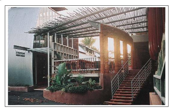
North and south wing run parallel to each other enclosing a cloistered garden terminating in a covered patio centre. The main dining room is on the right with reception offices on the left, with timber banisters used to connect hot dip galvanized steel hand rails (photo 2001).
