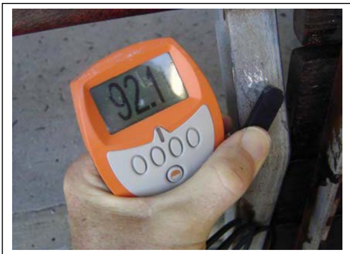
Typical measurement of a hot dip galvanized seat support bracket
