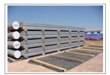
Hot dip galvanized air cooled condensers, stored on site, exposed to wet and dry atmospheres, for upwards of 12 months
