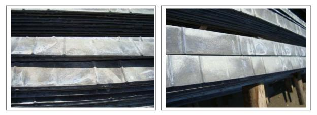
Removing the top strap from the stacked bundles of re-enforcing straps, the extent of the wet storage stain becomes evident
