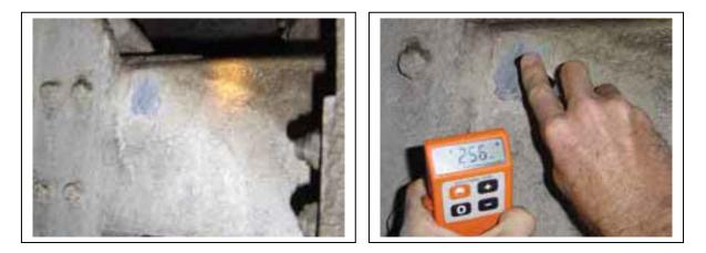
The coating thickness on shaft buntons at four different levels were inspected and found to be similar and were in a range of 250 to 300µm
