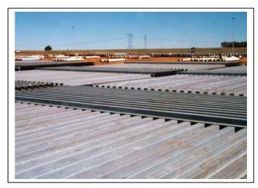
Hot dip galvanized shaft guides laid out at the mine waiting installation during the course of 1997
