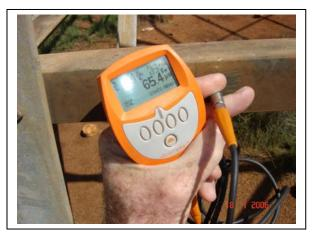
Site No. 1 After removing the "apparent" rust discolouration, the underlying zinc hot dip galvanized coating measured 65 $\mu$ m. Accuracy of the instrument is approximately 5%.
