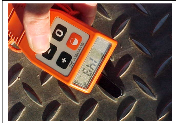
General view of the “Vastrap Plate” walkway that shows coating thickness adjacent to the anti-skid ridges of 149µm
