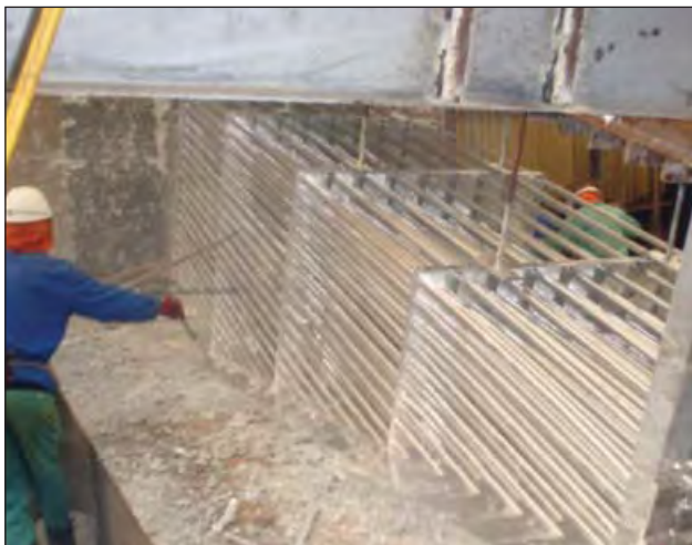
Hot dip galvanizing of cooling coils such as these must be forced into the molten zinc bath in order that only the outer surface of the tube be coated.
