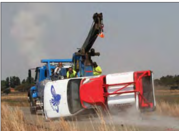
Finite Element Testing (FEA) was verified using physical tests including deliberately destroying a vehicle in a multiple roll.
