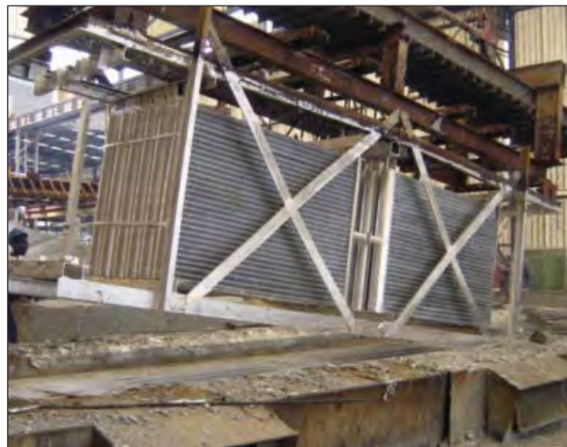
Hot dip galvanizing of cooling coils such as these must be forced into the molten zinc bath in order that only the outer surface of the tube be coated.
