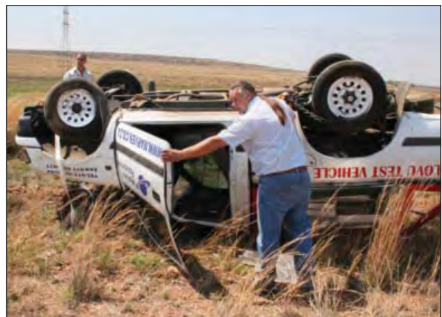
Finite Element Testing (FEA) was verified using physical tests including deliberately destroying a vehicle in a multiple roll.
