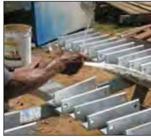
Duram duplex coating surface preparation: detergent wash and water rinse.
