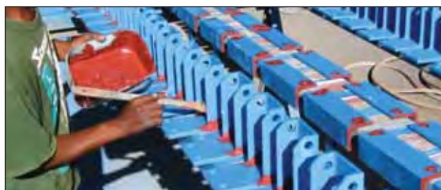
Duram products being applied directly using airless spray or brush application from the can without mixing or thinning and without runs or sags.
