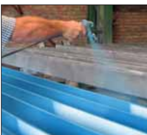
Duram products being applied directly using airless spray or brush application from the can without mixing or thinning and without runs or sags.
