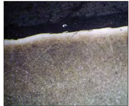
Figure 7. The mechanically plated coating in cross section (125x).
