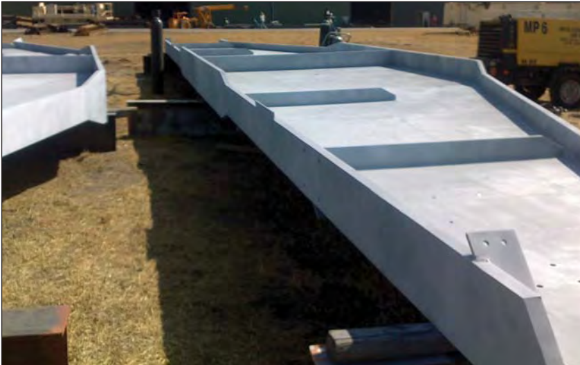
The appearance of the finished zinc metal sprayed coating.
