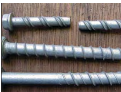
Figure 3. The mechanically plated samples as received, with all the fastener manufacturers represented.
