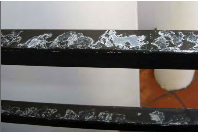
Delamination of the galvanizing due to shot blasting, usually results in complaints that the galvanizing was inadequate.
