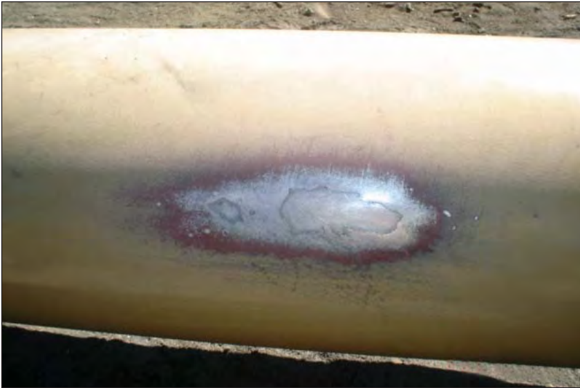
Delamination of the galvanizing due to shot blasting, usually results in complaints that the galvanizing was inadequate.
