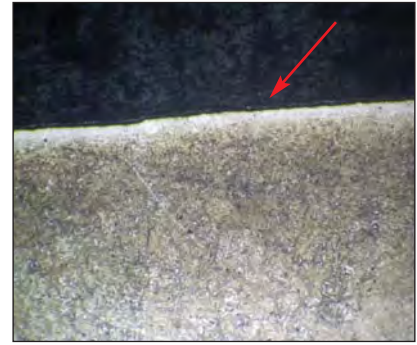
Figure 5. The electroplated coating in cross section (125x). Note the carburized surface skin of the substrate.
