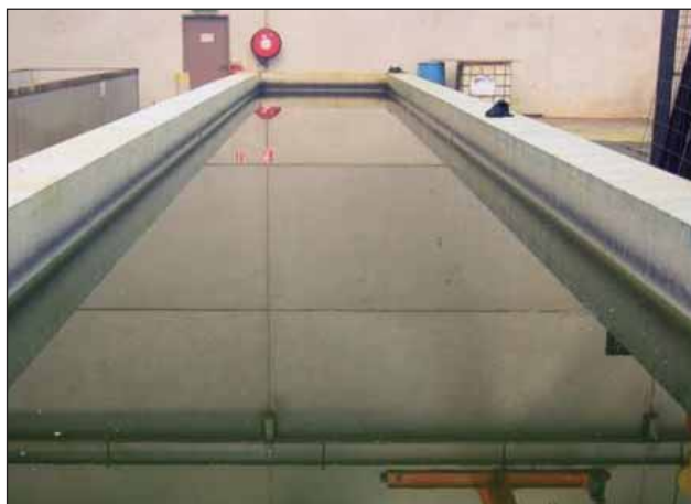
Low operating temperature of the new degreaser, considerably reduces the evaporation.
