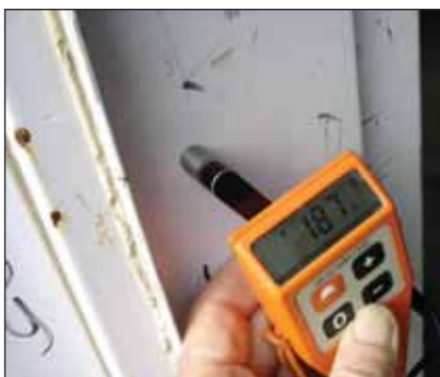
Photo above left, shows the overall coating thickness of the zinc electroplated and the powder coating (187µm). Photos above centre and right shows the general coating thickness of the zinc electroplating (13.1 and 4.7µm respectively).
