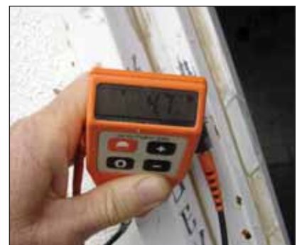
Photo above left, shows the overall coating thickness of the zinc electroplated and the powder coating (187µm). Photos above centre and right shows the general coating thickness of the zinc electroplating (13.1 and 4.7µm respectively).
