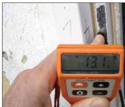
Photo above left, shows the overall coating thickness of the zinc electroplated and the powder coating (187µm). Photos above centre and right shows the general coating thickness of the zinc electroplating (13.1 and 4.7µm respectively).
