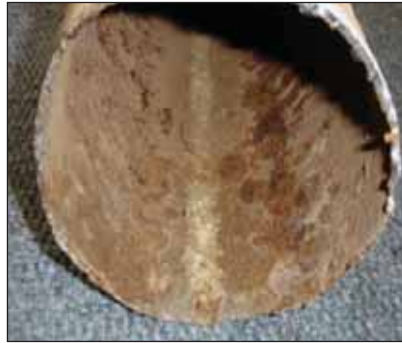
Sample pipe recovered from a 10-year-old centre pivot. Pipe was removed from service due to mechanical damage to the machine.
