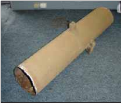
Sample pipe recovered from a 10-year-old centre pivot. Pipe was removed from service due to mechanical damage to the machine.
