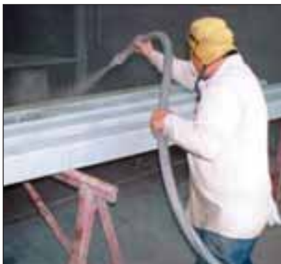
Sweep blasting at a blast pressure of less than 200kpa and correct angle removes the zinc corrosion products and roughens the surface to make a good profile for paint adhesion.
