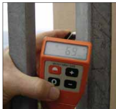
The pedestrian gate was installed in 2004 (left) and from coating thickness readings (right) the coating was hardly affected and in good condition. There were no signs of surface zinc chloride on the coating.
