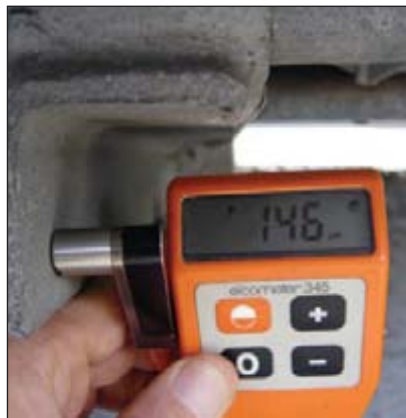
Coating thickness ranged from 117 to 146µm.
