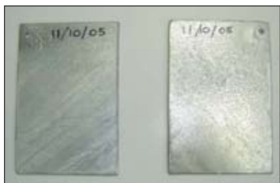
Coating thickness readings before sweep blasting: Left: Mean 111 Min 94 Max 141 No. of readings 15 Right: Mean 85 Min 73 Max 98 No. of readings 16
