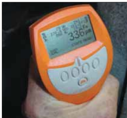
Photos 3 – 4 show the total coating thickness of the duplex coating system at 336µm and 378µm respectively.
