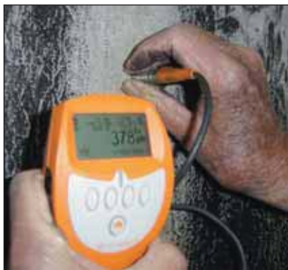
Photos 3 – 4 show the total coating thickness of the duplex coating system at 336µm and 378µm respectively.
