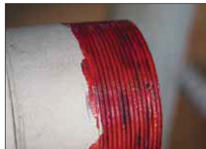
Photo below shows male threads coated with Galvstop and above where Galvstop has been removed after hot dip galvanizing in this female thread, showing purposely uncoated threads.
