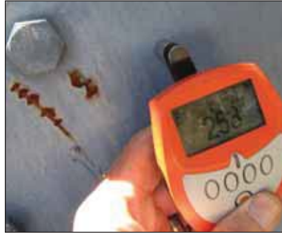
Painted ring and body showing signs of corrosion in spite of coating thickness of 253µm.
