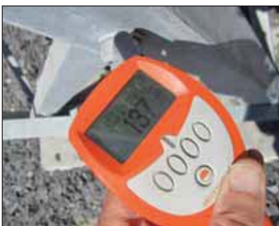
Hot dip galvanized nuts indicating a coating of 137 and 122 \mu m respectively
