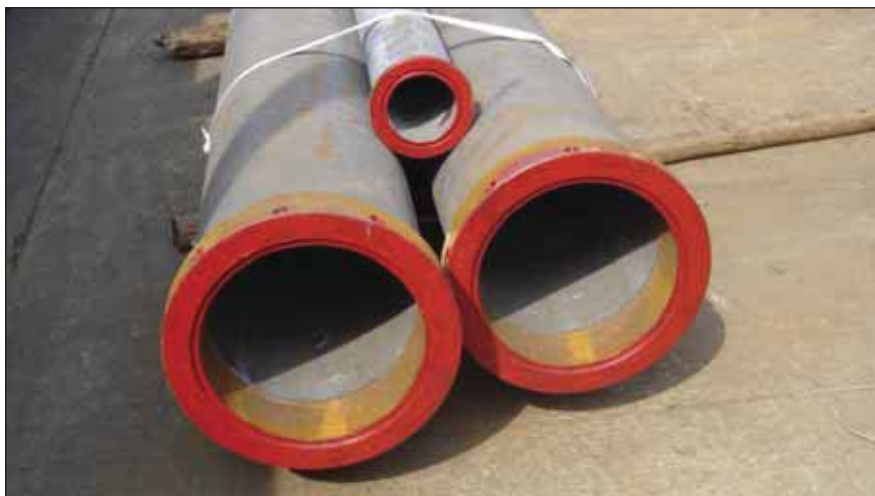
High pressure water pipes have close fitting couplings that can successfully clamp to optimally zinc metal sprayed pipe ends. Masking is used to exclude hot dip galvanizing.
