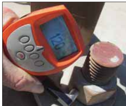
Hot dip galvanized nut on structure and holding down nut 77.3 and 120µm respectively.
