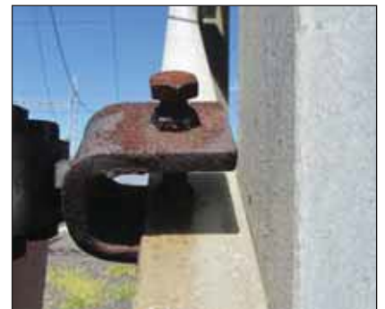
Uncoated or failed electroplated clamp.
