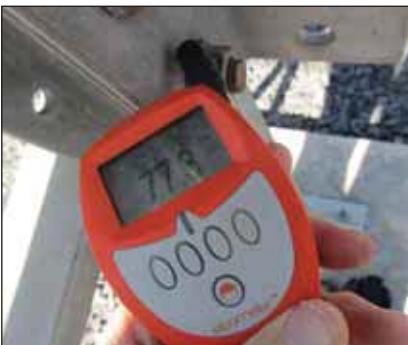
Hot dip galvanized nut on structure and holding down nut 77.3 and 120µm respectively.
