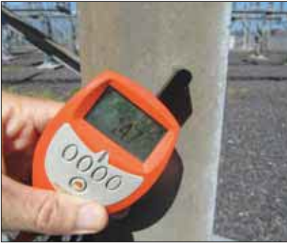
Above (left to right) and below (left and centre): Coating thicknesses taken on the transmission pylons of 143, 201, 146, 147 and 173µm respectively.
