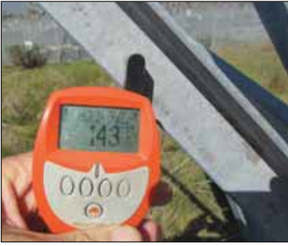
Above (left to right) and below (left and centre): Coating thicknesses taken on the transmission pylons of 143, 201, 146, 147 and 173µm respectively.
