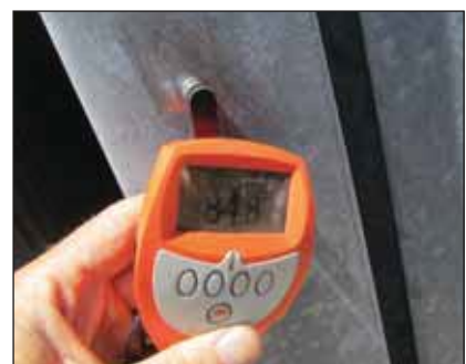
Hot dip galvanized radiator surface cleaned of surface contaminants and coating thickness readings of 83.8 and 84.8 \mu m respectively recorded.
