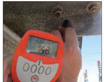
Electroplated nut 10.4µm.
