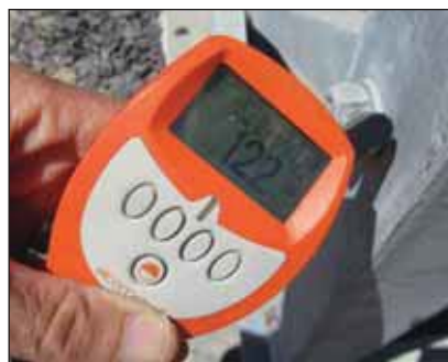
Hot dip galvanized nuts indicating a coating of 137 and 122 \mu m respectively
