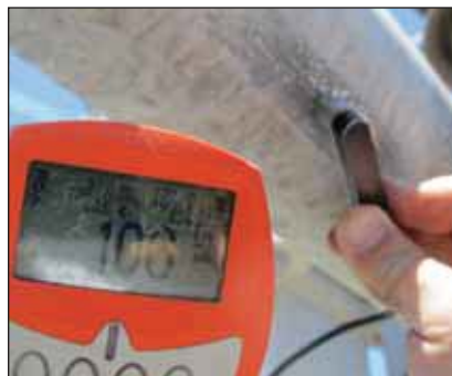
Hot dip galvanized tube cleaned of contaminants and coating thickness readings taken as 106 and 133µm respectively.
