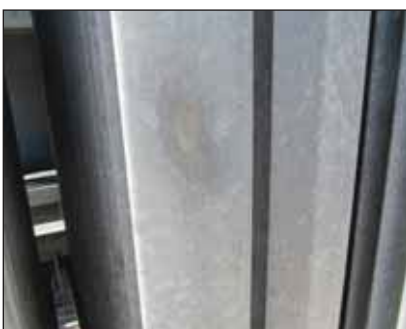
Hot dip galvanized radiator surface cleaned of surface contaminants and coating thickness readings of 83.8 and 84.8 \mu m respectively recorded.
