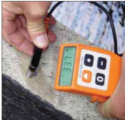
Photos 22 – 23: Total coating thickness 337µm and the hot dip galvanized coating thickness 123µm. Note the paint had to be removed to measure this.
