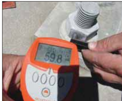
Hot dip galvanized nut 59.8µm.
