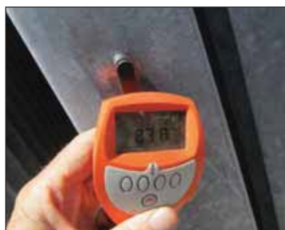
Hot dip galvanized radiator surface cleaned of surface contaminants and coating thickness readings of 83.8 and 84.8 \mu m respectively recorded.
