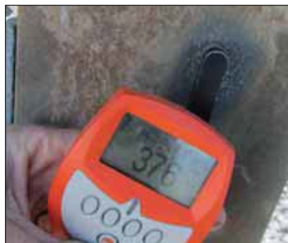
Discolored hot dip galvanized coating including coating thicknesses of 376 and 338µm respectively.
