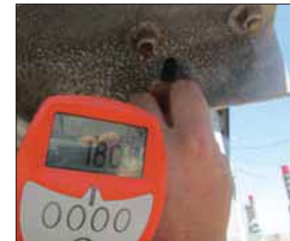
Coating contaminants removed and residual coating thickness measured 180 and 148µm respectively.
