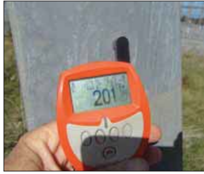
Above (left to right) and below (left and centre): Coating thicknesses taken on the transmission pylons of 143, 201, 146, 147 and 173µm respectively.
