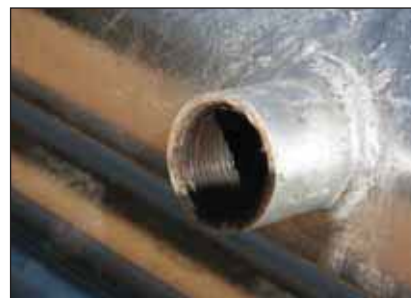
Photo below shows male threads coated with Galvstop and above where Galvstop has been removed after hot dip galvanizing in this female thread, showing purposely uncoated threads.
