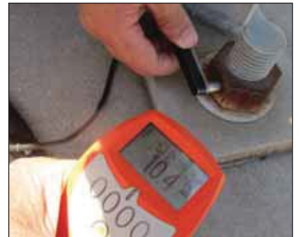
Electroplated nut 10.4µm.
