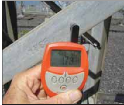
Above (left to right) and below (left and centre): Coating thicknesses taken on the transmission pylons of 143, 201, 146, 147 and 173µm respectively.
