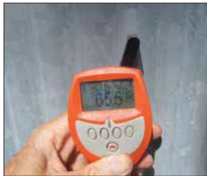
Hot dip galvanized radiators with coating thicknesses of 69.5 and 65.5µm respectively.
