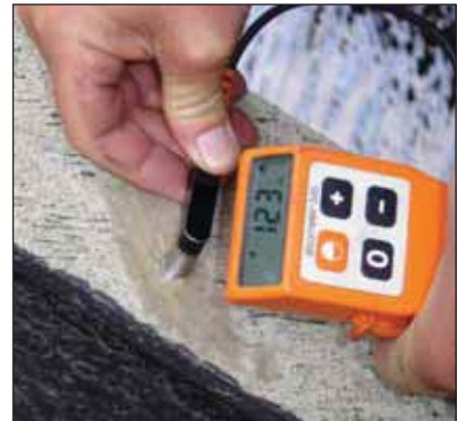
Photos 22 – 23: Total coating thickness 337µm and the hot dip galvanized coating thickness 123µm. Note the paint had to be removed to measure this.
