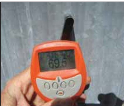
Hot dip galvanized radiators with coating thicknesses of 69.5 and 65.5µm respectively.
