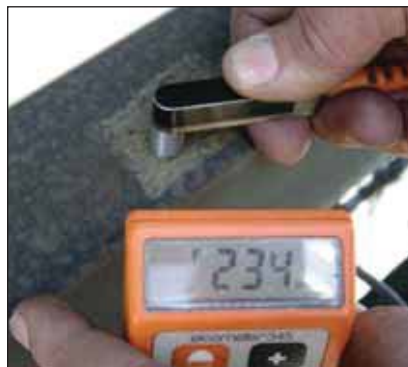
Photos 7 – 8 showing some typical coating thickness readings (298 and 234µm respectively).
