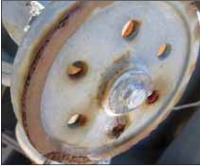
Painted ring and body showing signs of corrosion in spite of coating thickness of 253µm.
