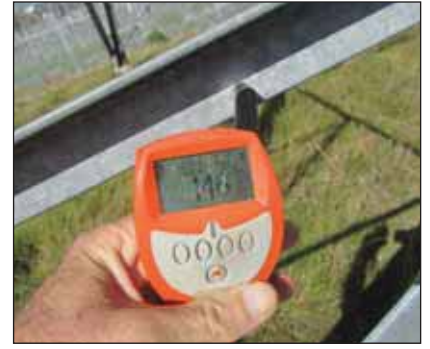
Above (left to right) and below (left and centre): Coating thicknesses taken on the transmission pylons of 143, 201, 146, 147 and 173µm respectively.
