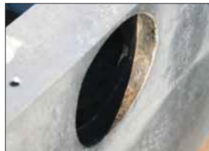
This hole inside has been coated with Galvstop and after hot dip galvanizing has been cleaned out, showing a purposely uncoated area.
