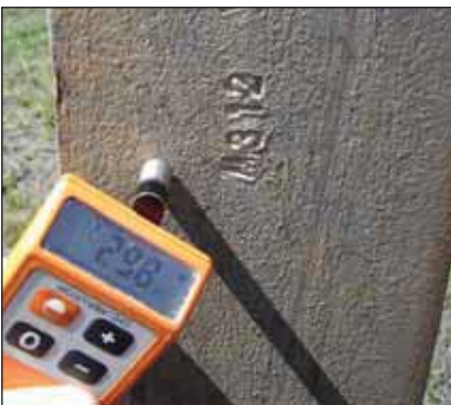
Photos 7 – 8 showing some typical coating thickness readings (298 and 234µm respectively).
