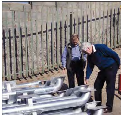
Inspecting a series of hot dip galvanized truck wheel guides prior to despatch to another client.
