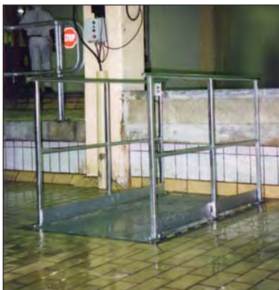
Hot dip galvanized Lifting Table, Clover Boksburg – in compliance with the new Food Safety Act and H.A.C.C.P.
