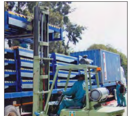
Duplex coated (hot dip galvanized and painted) dock levellers being loaded for despatch to Distribution Centre in Luanda Angola.
