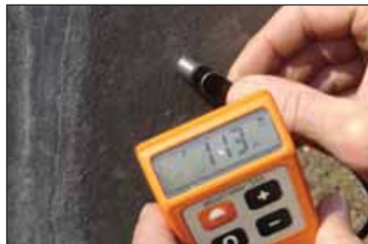
Photos above starting top left in each row show residual coating thickness readings of 90; 138; 142; 102; 48; 84; 85; 113 and 75 \mu\text{m} , taken on the 132/88kV terminal tower and one of isolator supports.
