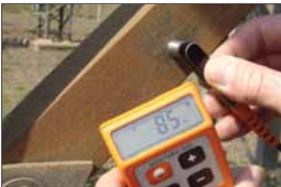
Photos above starting top left in each row show residual coating thickness readings of 90; 138; 142; 102; 48; 84; 85; 113 and 75 \mu\text{m} , taken on the 132/88kV terminal tower and one of isolator supports.
