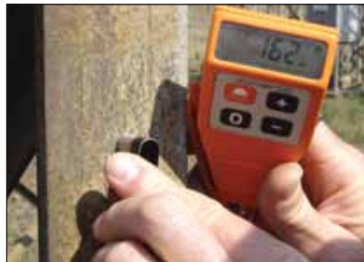
Photo right shows Mr Rob Maitland-Stuart of Eskom Distribution looking very satisfied at the thought of not having to refurbish the coating due to its substantial residual coating, see photo above left (162 \mu\text{m} ).
