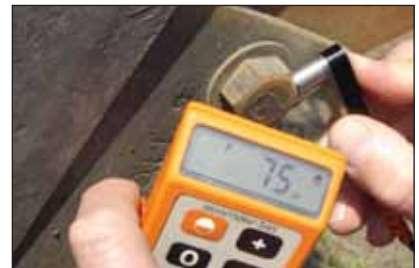
Photos above starting top left in each row show residual coating thickness readings of 90; 138; 142; 102; 48; 84; 85; 113 and 75 \mu\text{m} , taken on the 132/88kV terminal tower and one of isolator supports.
