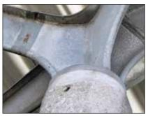
Due to the application thinness of Zincfix (achieveable by thinly spreading the product with one's finger) the welded area is showing signs of premature corrosion.
