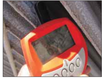
Above left and right: Residual coating thicknesses of 71.4 and 69.0µm respectively.
