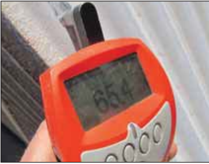
Above left and right: Residual coating thicknesses of 65.4 & 75.2µm respectively.
