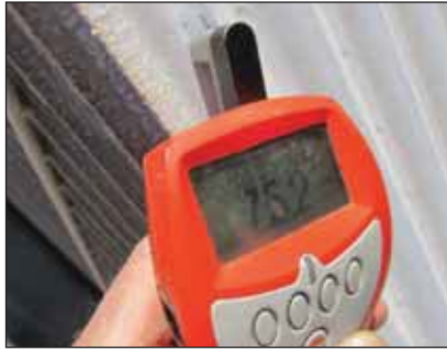
Above left and right: Residual coating thicknesses of 65.4 & 75.2µm respectively.
