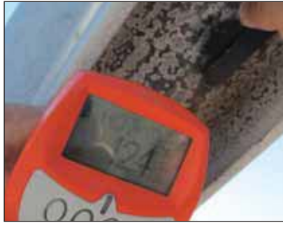
Above left, centre and right: Another component showing visible chloride salts, removed and residual coating thickness readings of 124 and 123 \mu m respectively.
