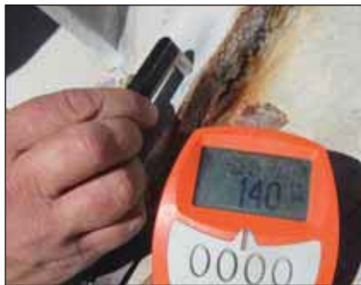
One single base plate showed corrosion on the edge. Residual coating thickness readings of 140 and 165 \mu m were taken adjacent to the corroded area. A possible cause is an original over cleaned edge or use of an acidic grout.
