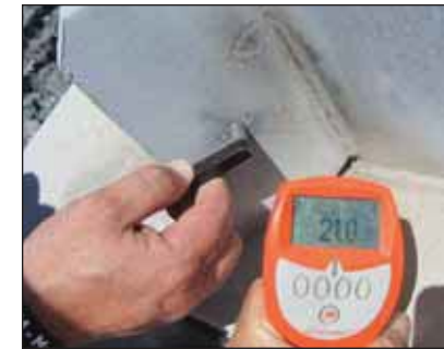
Above left, centre and right: Residual coating thicknesses adjacent to mechanical damage of 204µm, residual iron zinc alloy coating thickness at damage of 21.0 and 35.0µm respectively.
