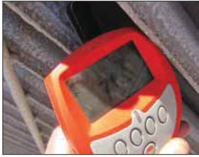
Above left and right: Residual coating thicknesses of 71.4 and 69.0µm respectively.
