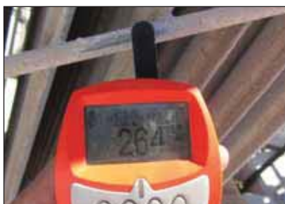
Above left and right: Residual coating thickness readings of 264 & 215µm respectively on the bracing struts.
