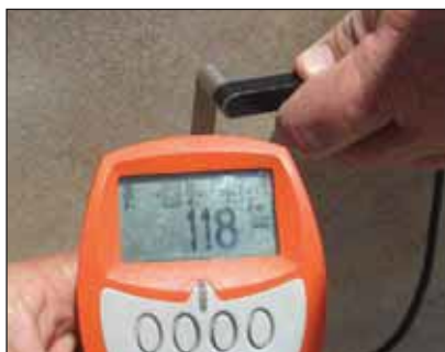
Above left and right: Coating thickness readings of 62.9 and 118 \mu m respectively on the topside of the duct cover plates.
