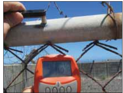
Coating thickness reading of 112 \mu m on the steel entrance gate.
