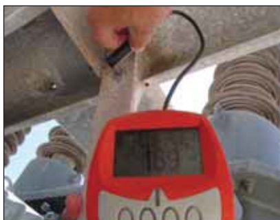
Above left, centre and right: Appearance of the coating on support angle, with residual coating thickness taken at a cleaned area of 169 and 191µm respectively.
