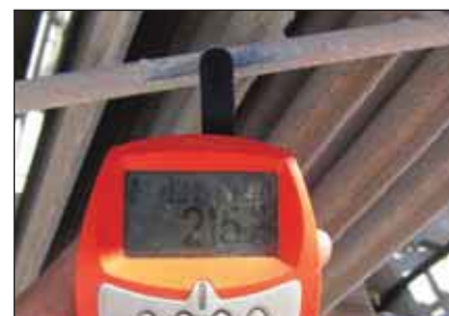
Above left and right: Residual coating thickness readings of 264 & 215µm respectively on the bracing struts.
