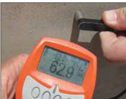
Above left and right: Coating thickness readings of 62.9 and 118 \mu m respectively on the topside of the duct cover plates.
