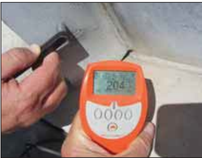
Above left, centre and right: Residual coating thicknesses adjacent to mechanical damage of 204µm, residual iron zinc alloy coating thickness at damage of 21.0 and 35.0µm respectively.
