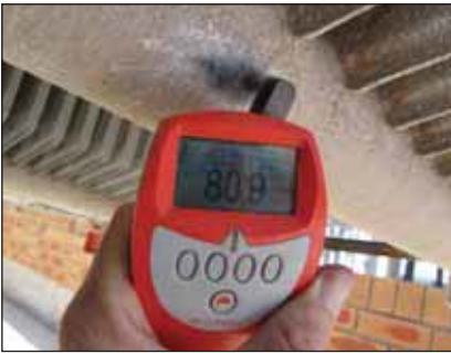
Above left and right: Residual coating thicknesses of 80.9 and 98.8µm respectively taken on the underside of the radiator.
