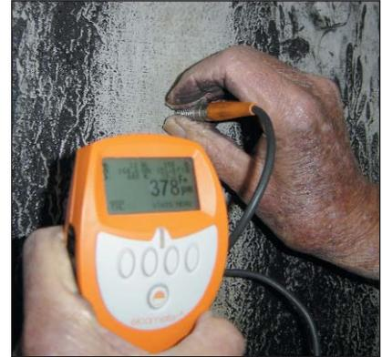
This 378 $\mu$ m coating reading was typical of that found on the structural steel.
