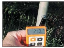
Photos 3 and 4 - Coating thickness readings on guard rail support (154 $\mu$ m) and balustrade transome (210 $\mu$ m) respectively.
