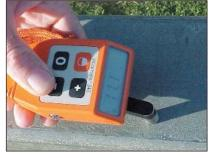
Photos I and 2- Coating thickness readings on the side (160 $\mu$ m) and top of the handrailings (171 $\mu$ m).
