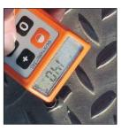
Photo 7 shows the close-up appearance of the "Vastrap Plate" and photos 8 and 9 show the coating thickness readings taken on the anti-skid ridges of the "vastrap plate" (11,6 to 140µm).
