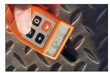
Photo 5 shows the general view of the "Vastrap Plate" walkway and photo 6 shows the general coating thickness, measured adjacent to the anti-skid ridges (149 $\mu$ m).
