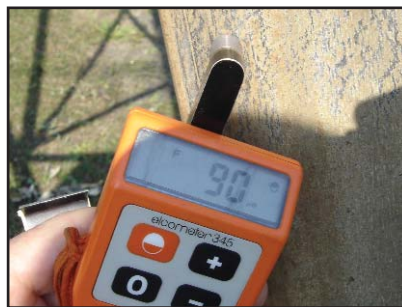
Photos 12 & 13: Residual coating thickness readings of 90 and 85µm, taken on the 132/88kV terminal tower and two of the isolator supports.
