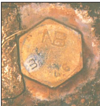
Figure 87. Galvanized bolt in contact with 3CR12 plate after 10 cycle SO 2 test. Note the cathodic protection provided by the galvanized bolt head to the surrounding steel.
