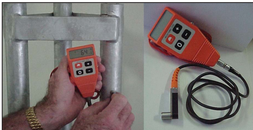
Figure 82. Using a digital instrument to measure zinc coating thickness.
