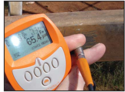
Photos 14 & 15: Site No. 1 – After removing "apparent" rust discolouration, the underlying hot dip galvanized coating measured 65.4µm.
