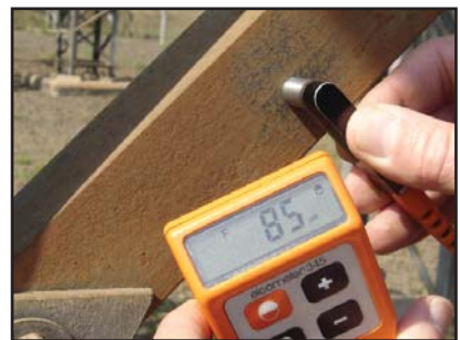
Photos 12 & 13: Residual coating thickness readings of 90 and 85µm, taken on the 132/88kV terminal tower and two of the isolator supports.
