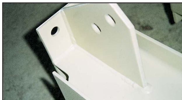
Figure 112. Sweep blasted hot dip galvanized coating followed by an appropriate paint system.
