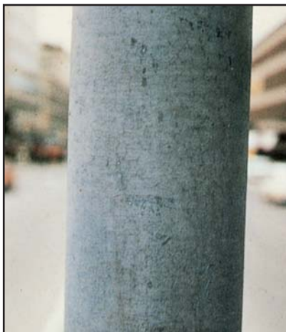
Figure 83. Exposed surface of a hot dip galvanized coating with outer layer of pure zinc. The shiny surface disappears to be replaced by grey corrosion products (sometimes called zinc patina).
