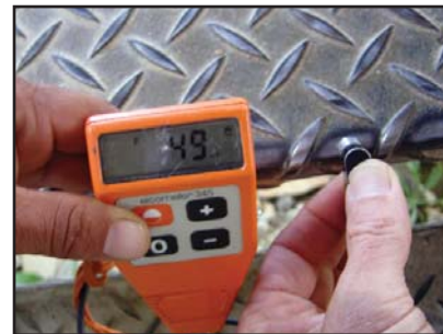
Figure 5. Abrasion resistance of hot dip galvanized vastrap stairs (coating thickness - 49\mu\text{m} , taken 10 years after installation).
