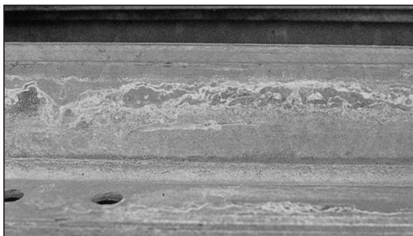
Figure 85. Wet storage stain that has formed between tightly packed angles.
