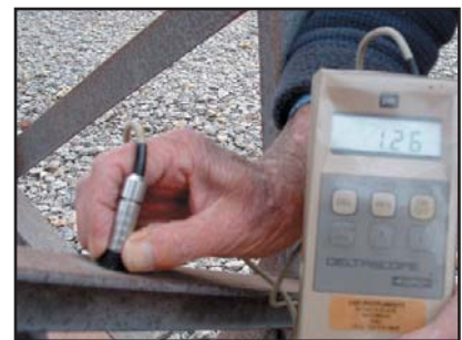
Photos 17 & 18: Despite the apparent "rust" contamination of the galvanized surface, once removed the galvanized coating measured 126µm.
