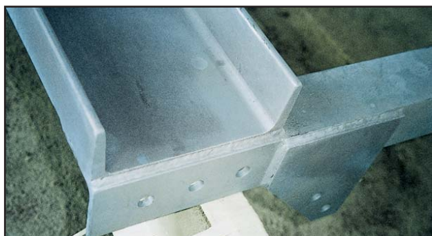
Figure 112. Sweep blasted hot dip galvanized coating followed by an appropriate paint system.
