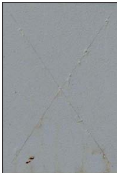
Powder coated continuous hot dip galvanized sheeting – Z275 – 2 000 hours salt spray.
