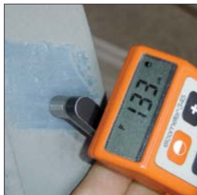
Total coating thickness reading on the cleaned up side rail of the cable ladder.
