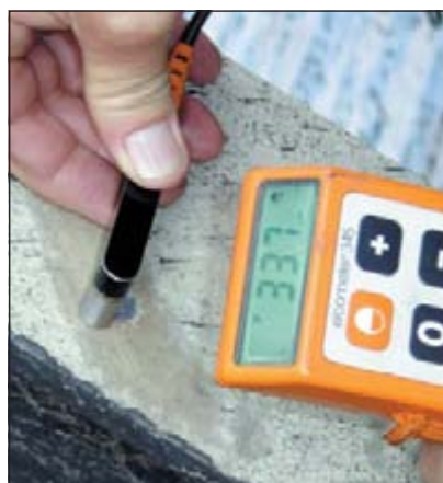
Total duplex coating thickness.
