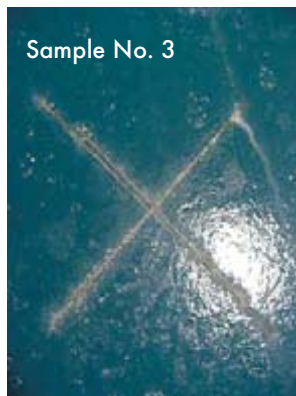
Comparison No. 2: Cross scribing after 4 000 hours salt spray exposure
