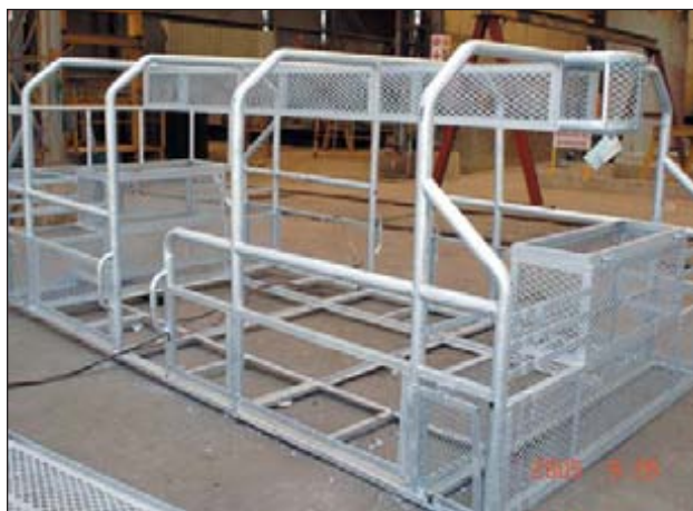
One of the first box frames to be hot dip galvanized in a single dip.
