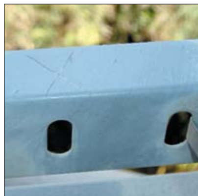
Exposed powder coating subjected to a cross cut adhesion test.
