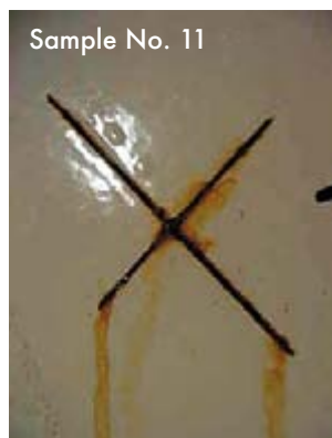
Comparison No. 1: Cross scribing after 4 000 hours salt spray exposure
