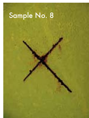
Comparison No. 2: Cross scribing after 4 000 hours salt spray exposure
