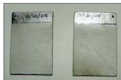
Coating thickness readings after sweep blasting: Left: Mean 121 Min 99 Max 148 No. of readings 15 Right: Mean 100 Min 84 Max 125 No. of readings 16
