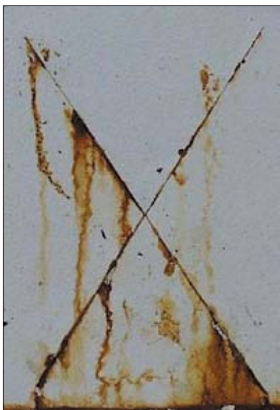
Powder coated mild steel – 2 000 hours salt spray.
