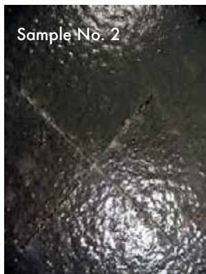
Comparison No. 1: Cross scribing after 4 000 hours salt spray exposure
