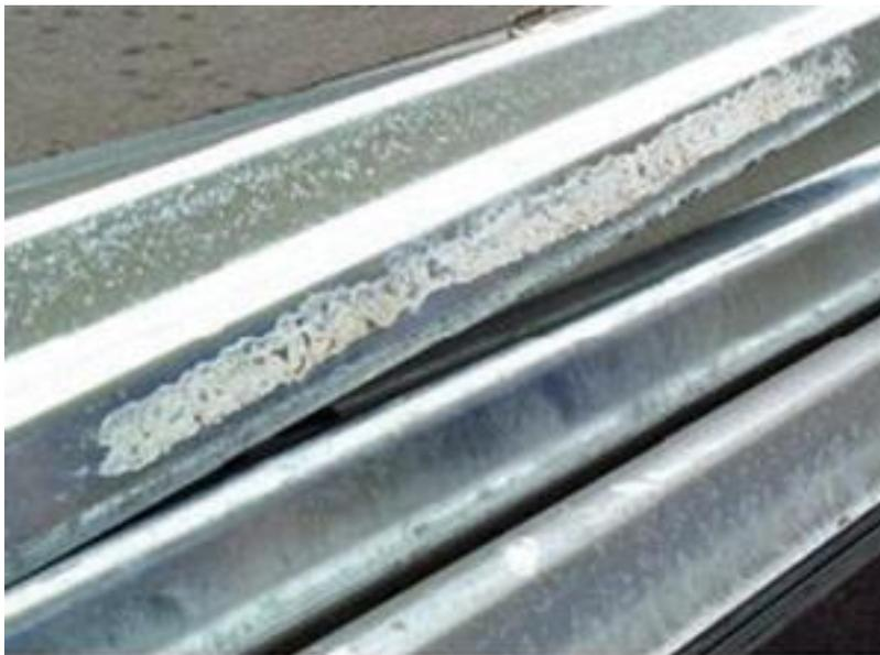
White-rust on a galvanized section of guard rail as a result of being tightly nested and stored in wet conditions
