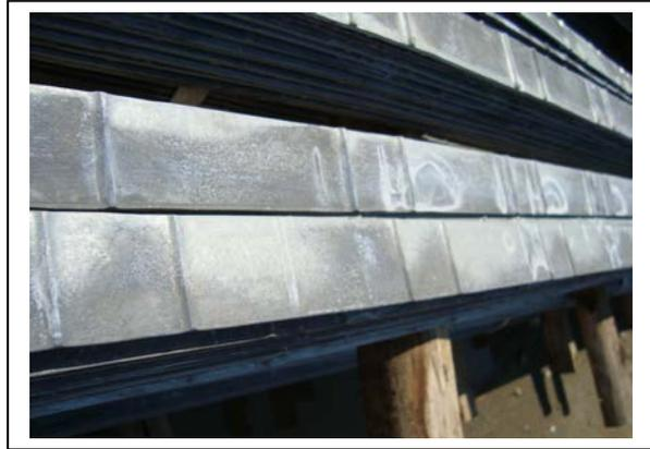
Removing the top strap from the stacked bundles of re-enforcing straps, the extent of the wet storage stain becomes evident
