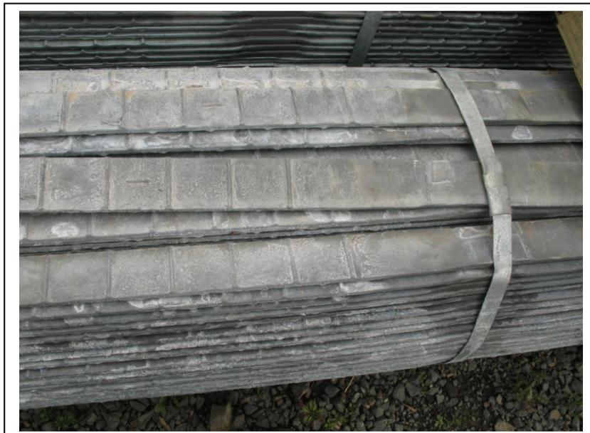
**Closely packed hot dip galvanized strips stored with water trapped within the bundles**
