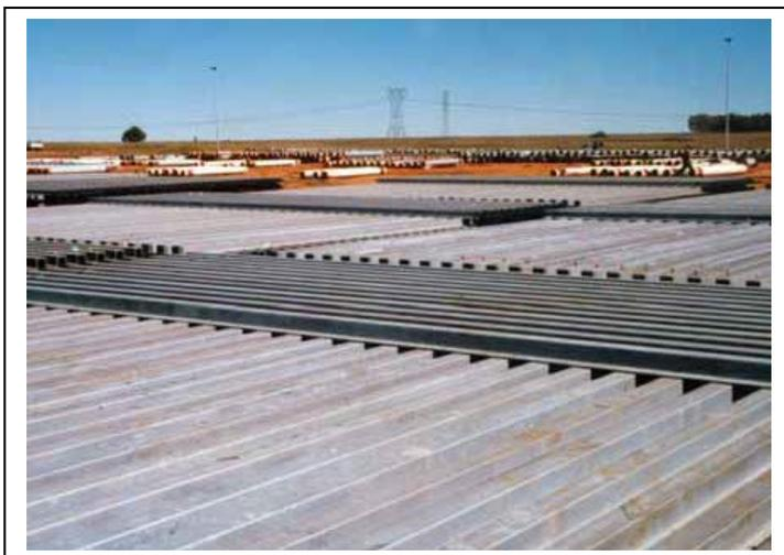
**Hot dip galvanized shaft guides laid out at the mine waiting installation during the course of 1997**
