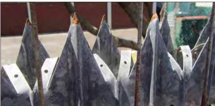
The above photo shows the thinly galvanized coating (Z275) (used for security spikes in Kenilworth Cape Town after about 15 years of exposure) being a minimum of 13.5µm to a nominal 20µm per face (when new), both the edges and more so at the tip, the zinc coating providing CP will slowly recede away from the edge or tip revealing a localised rusted area, which as the zinc recedes, will gradually increase in size.
