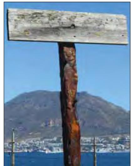
Inadequate corrosion specification.
