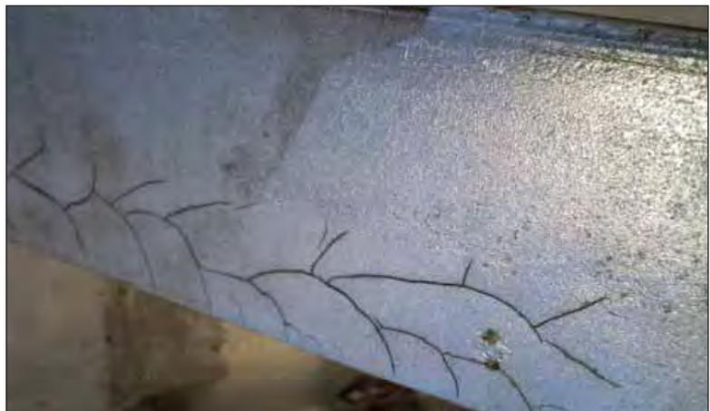
Out of spec. high levels of phosphorous can cause severe cracking of the coating.
