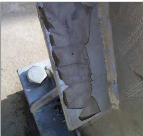
Cracking of the coating caused by high levels of phosphorous can cause follow on coating delamination.
