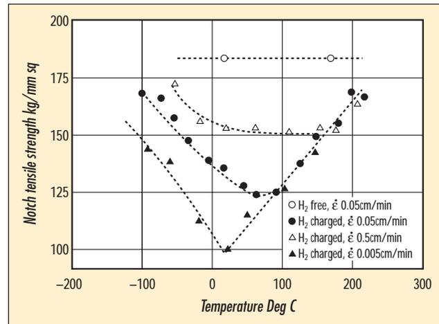
Figure 1.6.2.1: The notched tensile strength of steel AISI 4340 as a function of test temperature for three strain rates of testing<sup>(8)</sup>.
