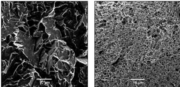
Figure 1.6.3.2: SEM fractographs of both cleavage and dimple fracture areas from the same freshly impact broken sample of a quenched and tempered low alloy Cr-Ni-Mo-V steel that was known to contain Hydrogen in excessive quantities. The white arrows show a few of the large number of secondary microcracks<sup>(9)</sup>.
