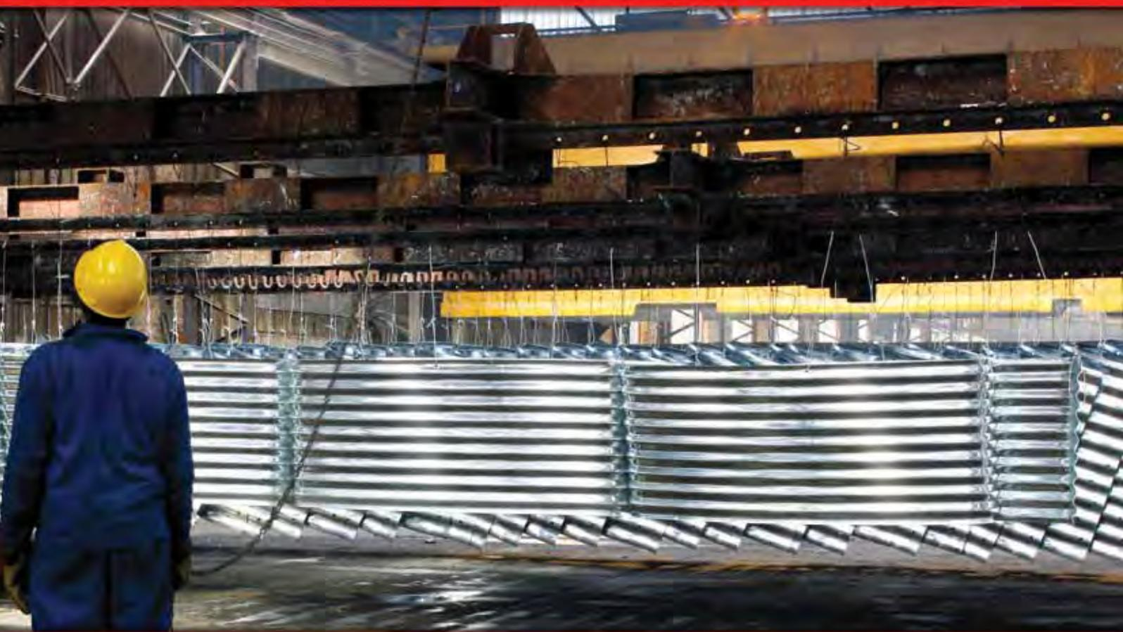
Our Isando plant can accommodate heavy steel structures due to our 13,2 meter kettle and improved crange and loading facilities.
