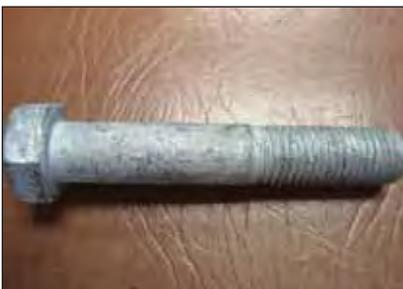
Photo 2: Rough surface finish usually the result of steel chemistry that increases the reactivity when immersed into molten zinc.
