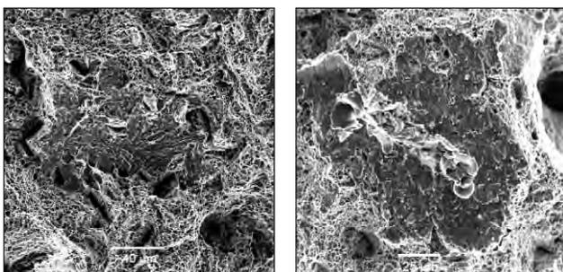
Figure 1.6.3.3: Slow SSR tested fractographs of the same 360mm shaft as in Figure 1.6.3.2 above. Note the "patches" of cleavage fracture areas amidst dimple fractured areas in the center of both figures with both of them showing clear "tear ridges"<sup>(10)</sup> seen as the fine lines on the cleavage planes<sup>(9)</sup>.
