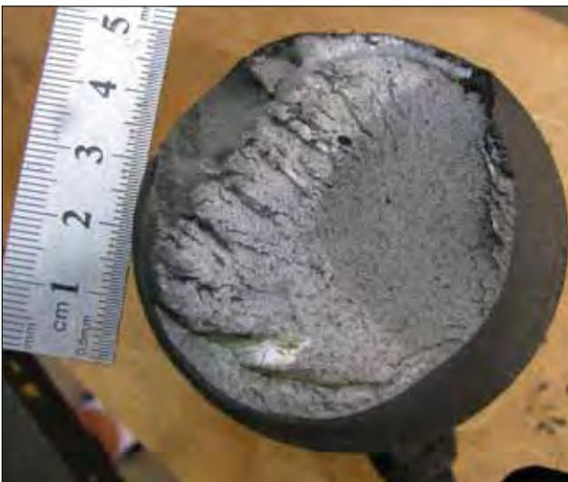
Figure 1: Overload fracture extending from the fatigue cracked zone (dark sickle-shaped region).
