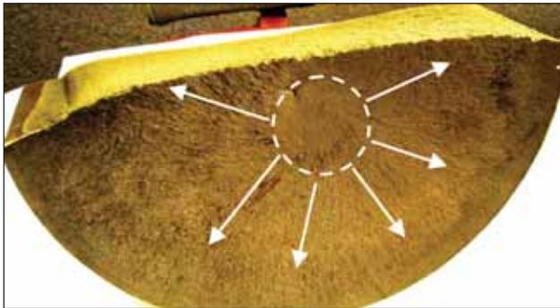
Figure 1.6.3.1: Macro-photographs of the failure by HE initiated at a "fish eye" of a 360 mm shaft manufactured from a low alloy Cr-Ni-Mo-V quenched and tempered steel<sup>(9)</sup>.
