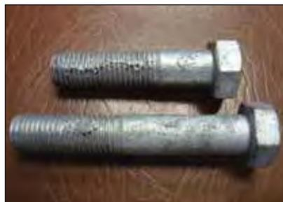
Photo 3: Bolt threads not cleaned and as such are not in conformance with the specification. Such components are rejectable and should be returned to the responsible galvanizer.
