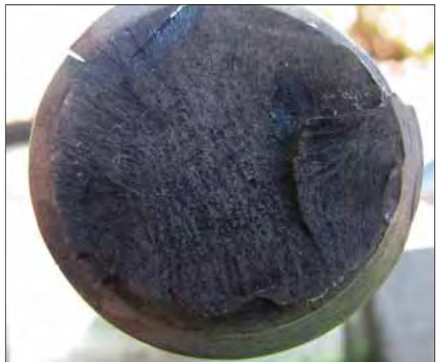
Figure 2: Bolt failure morphology ascribed to hydrogen assisted cracking (HAC).
