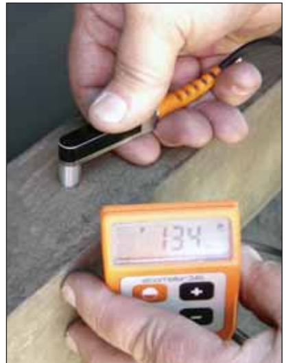
Coating thickness readings taken on all the horizontal and vertical overland conveyor steelwork were still in excess of that required by the specification.
