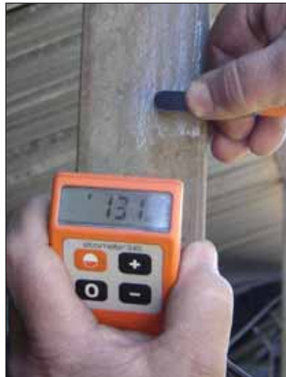
Coating thickness readings taken on all the horizontal and vertical overland conveyor steelwork were still in excess of that required by the specification.
