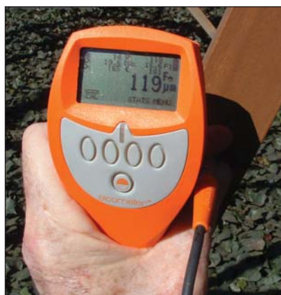
Site No 2. After the removal of the discoloration, i.e. corrosion products, the hot dip galvanized coating thickness measured to be 119µm.
