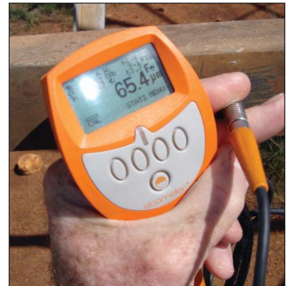
Site No 1. – After removing the “apparent” rust discoloration, the underlying hot dip galvanized coating measured 65,4µm. Accuracy of the instrument is approximately 5%.
