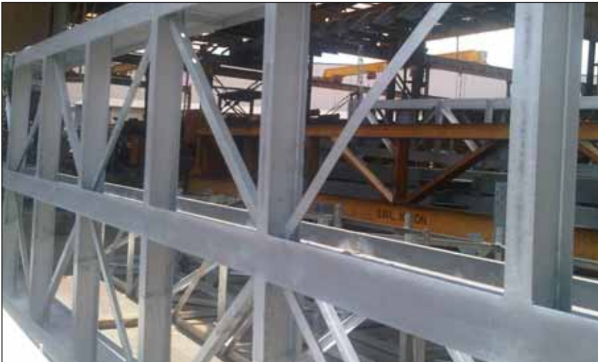
Figure 1a: Hot dip galvanized walkway platform with severely distorted 50 x 50 x 4mm angle section chords. Cracks were discovered after hot dip galvanizing at a number of the welded connections at the ends of the angle section chords. The angle sections had been welded to the 90° corner between the I-beam chords as shown in the left image in Figure 1b.
