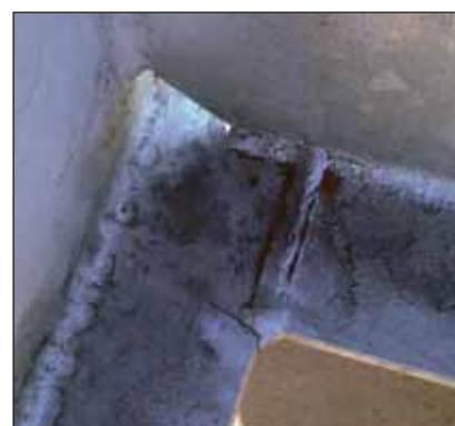
Figure 1d: Examples of cracks that had developed in I-beam flanges from 90° corners at T-joints between I-beam flanges.
