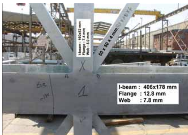
Figure 2a: The left image shows the new walkway platform with the design of the connections between the diagonal angle section chords and the I-beam chords modified. This is the first walkway platform that had been hot dip galvanized after the modification of the connection design. Cracks were discovered at a number of the welded connections between the 50 x 50 x 4mm diagonal angle section chords and the webs of the transverse 160 x 82mm I-beam chords at opposite sides of the middle longitudinal 406 x 178mm I-beam.
