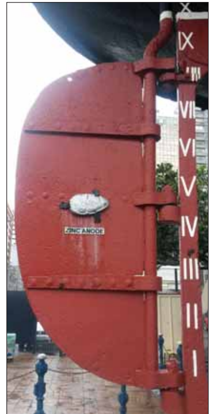
Sacrificial anodes electrically connected (bolted) to the carbon steel hull of a ship.
