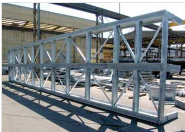
Figure 2a: The left image shows the new walkway platform with the design of the connections between the diagonal angle section chords and the I-beam chords modified. This is the first walkway platform that had been hot dip galvanized after the modification of the connection design. Cracks were discovered at a number of the welded connections between the 50 x 50 x 4mm diagonal angle section chords and the webs of the transverse 160 x 82mm I-beam chords at opposite sides of the middle longitudinal 406 x 178mm I-beam.
