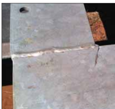
Figure 1d: Examples of cracks that had developed in I-beam flanges from 90° corners at T-joints between I-beam flanges.
