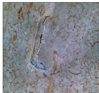
Figure 1c: Some of the angle section chords had fractured completely in the base metal some distance from the fillet welds and weld heat affected zones (left). The image on the right shows cracks that had penetrated the web of an I-beam chord at the fillet welded connection between the angle section chord and web of the I-beam chord at the opposite side. The failure of the angle section chord in the top image is similar to the LMAC failure of a diagonal chord on girder reported by CROSS in the United Kingdom. [CROSS (Confidential Reporting on Structural Safety), "Liquid Metal Assisted Cracking (1)", Report ID: cross45, Published: Newsletter No 4 - November 2006, http://www.structural-safety.org/view-report/cross46 ].
