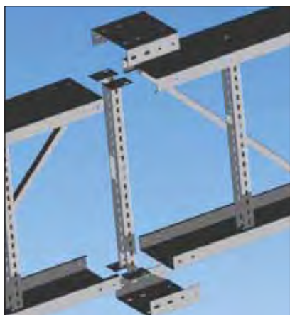
The splice is designed to be placed anywhere in the span.
