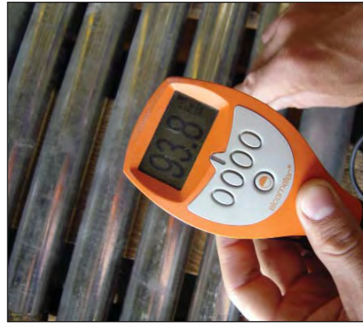
Photos above from left to right show the hot dip galvanized coating thickness to SANS 32 (EN 10240) (91.8; 93.8 and 71.0µm respectively) on the lower batch of tube in comparison.
