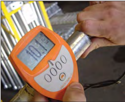
Clockwise from top left shows the outer upper coating thickness (22.3µm), the outer lower coating thickness (13.9µm), the inner lower coating thickness (4.9µm) and the inner upper coating thickness (10.1µm).
