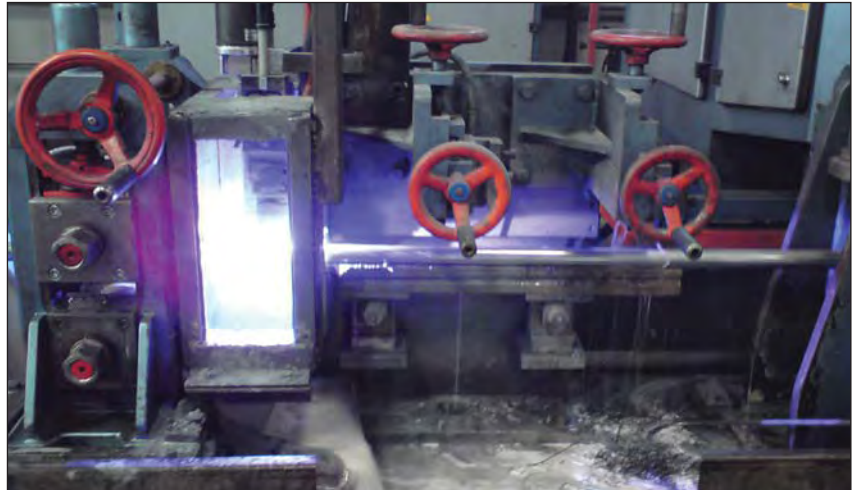
The weld repair system taking place in the spray chamber:
