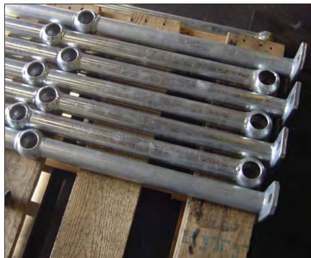
Hot dip galvanized tube to SANS 32 (EN 10240) and thinly zinc coated tube. Hot dip galvanized stanchions to SANS 121 (ISO 1461).
