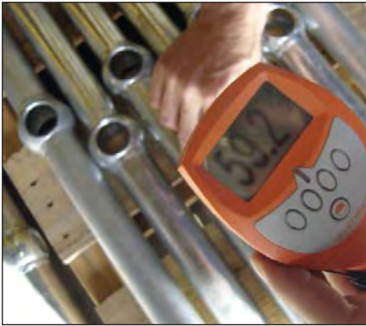
Photos above show the hot dip galvanized coating thickness on the stanchions (59.2 and 74.6µm). This is normal as per the requirement of SANS 121 (ISO 1461).
