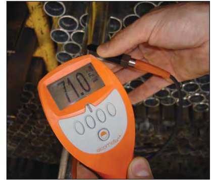
Photos above from left to right show the hot dip galvanized coating thickness to SANS 32 (EN 10240) (91.8; 93.8 and 71.0µm respectively) on the lower batch of tube in comparison.
