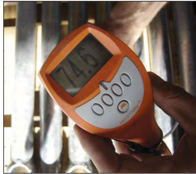
Photos above show the hot dip galvanized coating thickness on the stanchions (59.2 and 74.6µm). This is normal as per the requirement of SANS 121 (ISO 1461).
