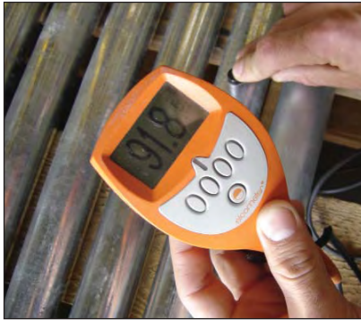
Photos above from left to right show the hot dip galvanized coating thickness to SANS 32 (EN 10240) (91.8; 93.8 and 71.0µm respectively) on the lower batch of tube in comparison.
