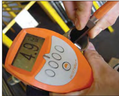
Clockwise from top left shows the outer upper coating thickness (22.3µm), the outer lower coating thickness (13.9µm), the inner lower coating thickness (4.9µm) and the inner upper coating thickness (10.1µm).
