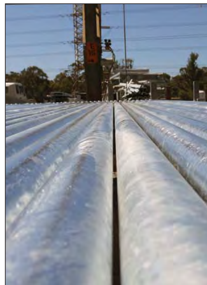
The bright, white rust free surface finish of non-reactive hot dip galvanized steel.
