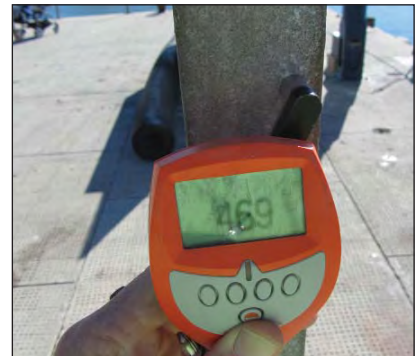
Zinc chloride layer including the hot dip galvanized coating thickness of 469 \mu m.
