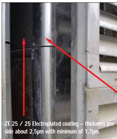
Z275 class of coating – coating thickness about 20µm with minimum of 13,5µm.
