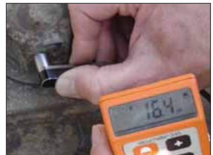
The paint support barrier over the HD nuts was easily removed and the residual zinc electroplated coating measured between 7.1 and 16.4 \mu\text{m} .
