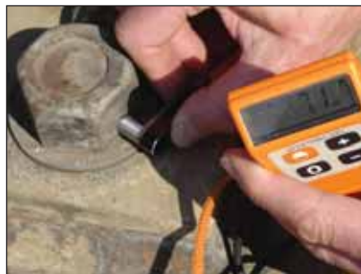
The paint support barrier over the HD nuts was easily removed and the residual zinc electroplated coating measured between 7.1 and 16.4 \mu\text{m} .
