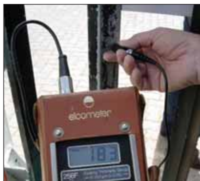
Photo left shows the overall coating thickness and right the hot dip galvanized coating thickness, suggesting that the paint coating was a DFT of about 40 odd micrometres.
