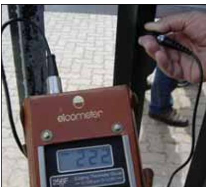
Photo left shows the overall coating thickness and right the hot dip galvanized coating thickness, suggesting that the paint coating was a DFT of about 40 odd micrometres.
