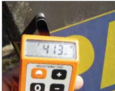
Coating thickness readings prove that the coating will provide a further 20 to 30 years of maintenance free life.
