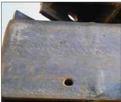
The surface profile of the black steel has resulted in striations in the hot dip galvanized coating – see photo below.
