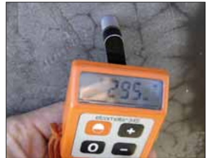
Coating thickness readings prove that the coating will provide a further 20 to 30 years of maintenance free life.
