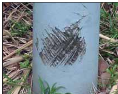
Photo 4: GRP light post where outer fibres have been exposed in the premature breakdown of the pole.
