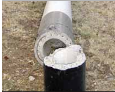
Photo 9: Concrete poles can fail with side impact loads.
