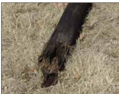
Photo 1: Without the correct treatment timber light poles can rot at the base.
