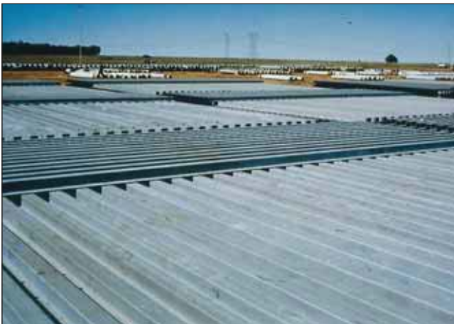
Hot dip galvanized shaft guides prior to installation into a deep level gold mine.
