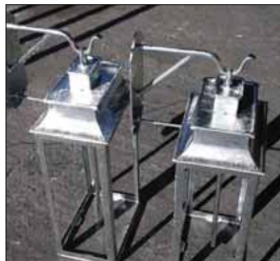
Left: Before nickel tablets. Right: Chrome like finish achieved after the addition of nickel tablet.
