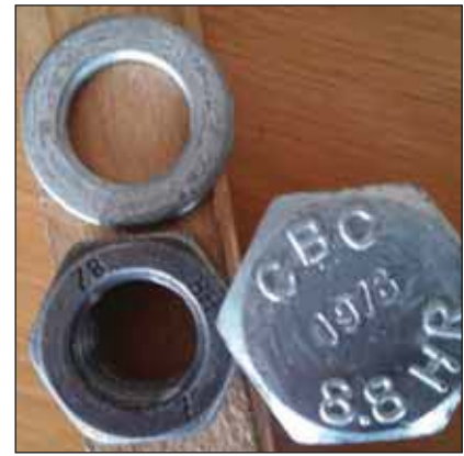
The nut is pre lubricated thus giving it an apparent different finish to the traditional hot dip galvanized finish which is on the bolt and washer.
