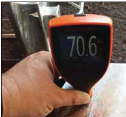
Thickness test done before the conversion to nickel tablets.
