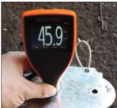
Drastic reduction achieved on an identical item dipped after the conversion with nickel tablets. Coating still within ISO specification.
