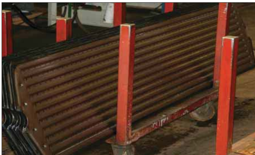
The 1mm thick cold formed pressed panels are inverted 180° against another panel and continuously welded on all the edges making up a complete radiator fin.
