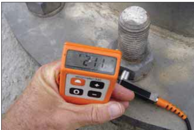
Photos 3 and 4: Coating thickness on the holding down nut 211 \mu m and on the mast 159 \mu m respectively.
