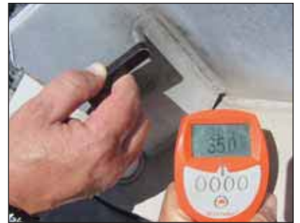
Above left, centre and right: Residual coating thicknesses adjacent to mechanical damage of 204µm, residual iron zinc alloy coating thickness at damage of 21.0 and 35.0µm respectively.
