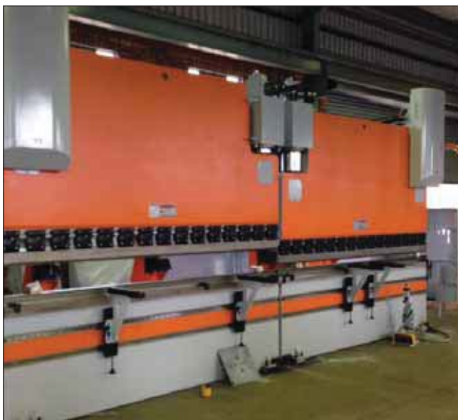
CNC press brake being commissioned at IPM.
