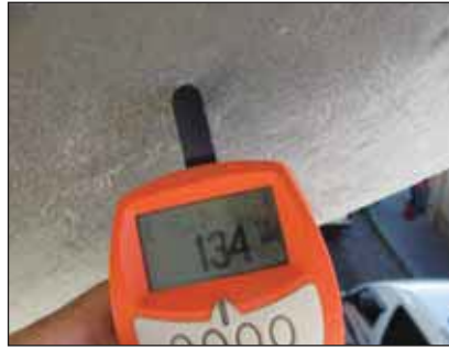
The curved hot dip galvanized tubular purlins are in excellent condition with a residual hot dip galvanized coating thickness of 134µm.
