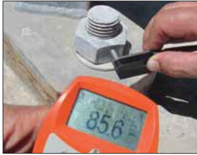
Above left, centre and right: Residual coating thickness readings on cleaned holding down nuts and bolts of 79.1, 85.6 and 260 \mu m respectively.
