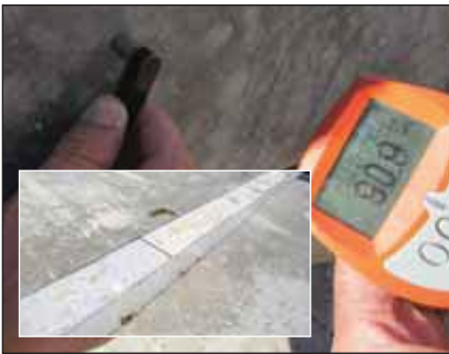
Insert showing galvanized steel duct cover plates. Above left and right: Coating thickness readings of 90.9 and 108 \mu m respectively on the underside of the duct cover plates.
