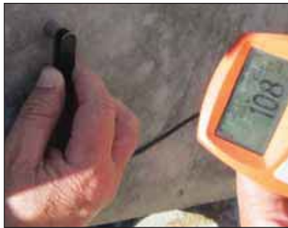
Insert showing galvanized steel duct cover plates. Above left and right: Coating thickness readings of 90.9 and 108 \mu m respectively on the underside of the duct cover plates.
