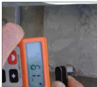
Photos 11 – 14 from top left clockwise: After 5 years of service at Bafokeng-Rasimone PCP – The appearance of the 3 coat paint system; a damaged hot dip galvanized coating; coating thickness on a hot dip galvanized water pipe (59µm) (tube hot dip galvanized to EN 10240) and coating thickness at the damaged area (61µm).
