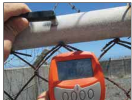
Coating thickness reading of 61.2 \mu m on the steel entrance gate.
