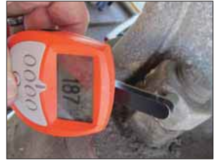
The surface contamination removed and residual coating thickness of 197µm taken on the structure and 187µm on the holding down nut.
