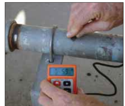
Photos 11 – 14 from top left clockwise: After 5 years of service at Bafokeng-Rasimone PCP – The appearance of the 3 coat paint system; a damaged hot dip galvanized coating; coating thickness on a hot dip galvanized water pipe (59µm) (tube hot dip galvanized to EN 10240) and coating thickness at the damaged area (61µm).
