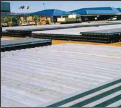
The shaft provides continual access for men, materials, machinery and ore, maintenance free performance of upwards of 25 years and is required to minimise routine downtime allowances. Photos 5 and 6 show hot dip galvanized shaft guides (left) and buntons and connections (right). Note the additional paint coating at crevices and over the fasteners.
