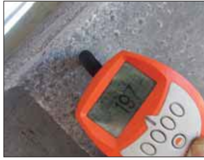
The surface contamination removed and residual coating thickness of 197µm taken on the structure and 187µm on the holding down nut.
