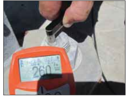
Above left, centre and right: Residual coating thickness readings on cleaned holding down nuts and bolts of 79.1, 85.6 and 260 \mu m respectively.
