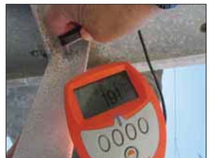
Above left, centre and right: Appearance of the coating on support angle, with residual coating thickness taken at a cleaned area of 169 and 191µm respectively.
