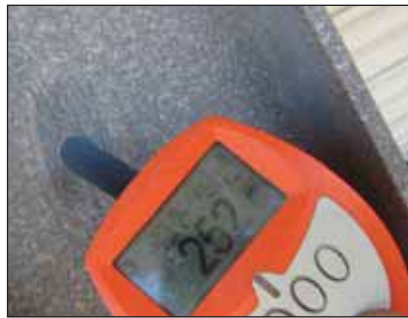
Hot dip galvanized I-Beam tubular purlin support, showing a residual coating thickness of 252µm.
