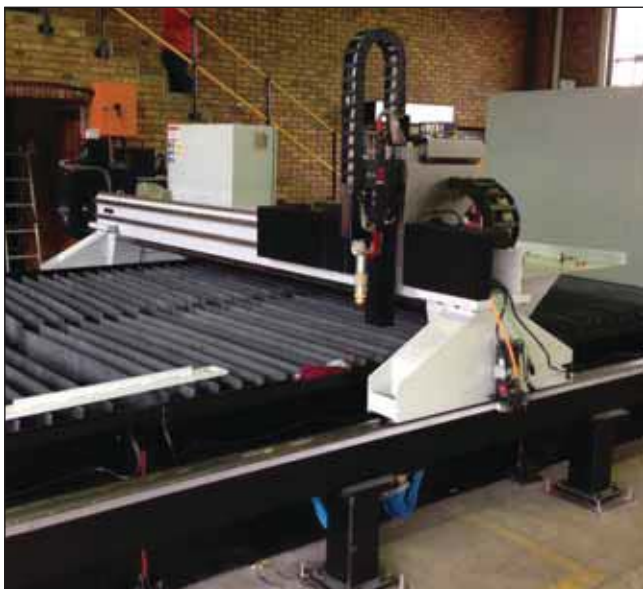
CNC plasma cutting machine is being commissioned at IPM.
