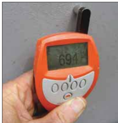
Close-ups showing the colour and coating thickness.
