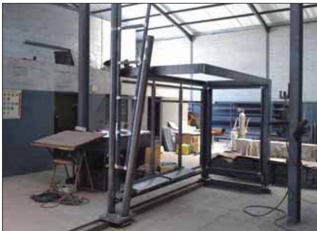
Two different bus shelter types at the fabricators plant, prior to hot dip galvanizing.
