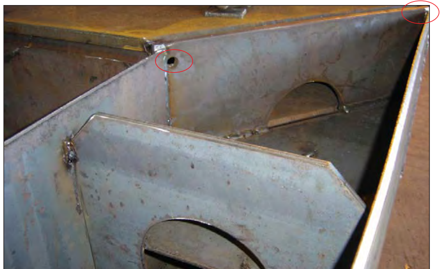
Photo 36. Increase vent, fill and drainage holes to as big as possible at the haunch plate.
