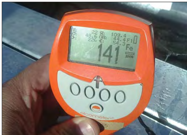
Photos above show S355 tube (open on both ends) hot dip galvanized at 450°C.
