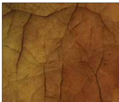
Figure 2: Rust stains on the resin face (left) with the chopped glass strands on the reverse face.
