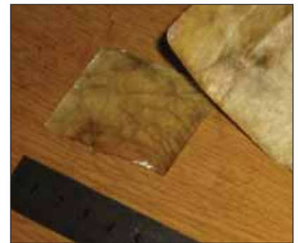
Figure 1: Glass reinforced polymer roofing section as received.
