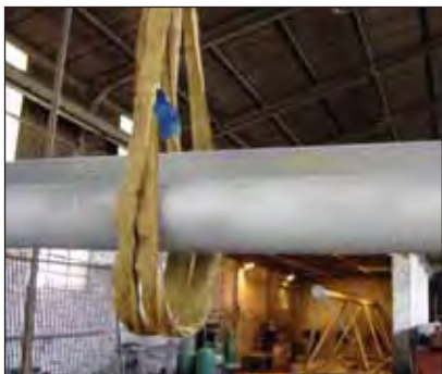
Photo 2: In order to minimise coating damage, only soft slings were used for loading/unloading for the duration of this project.
