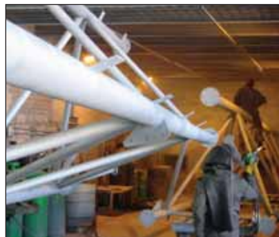
Photos 3 (left) and 4 (right) show the degree of difficulty in ensuring a uniform spread of zinc metal spraying to the specified coating thickness.
