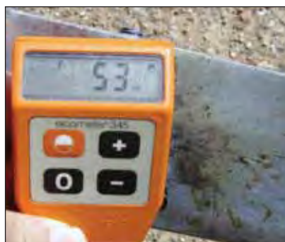
Photo 20 (above left) shows the coating thickness adjacent to the weld and photo 21 (above right) shows the coating thickness at weld area. Welding has visibly reduced the coating thickness.
