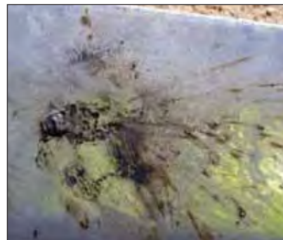
Photos 18 (above left) shows the weld mark as is, photo 19 (above right) shows all welding residues removed by scrapping.
