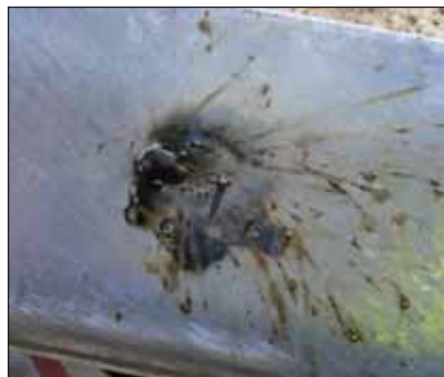
Photos 18 (above left) shows the weld mark as is, photo 19 (above right) shows all welding residues removed by scrapping.
