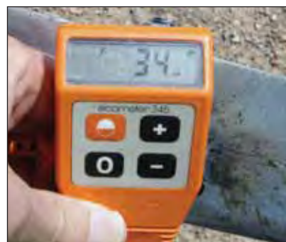
Photo 20 (above left) shows the coating thickness adjacent to the weld and photo 21 (above right) shows the coating thickness at weld area. Welding has visibly reduced the coating thickness.
