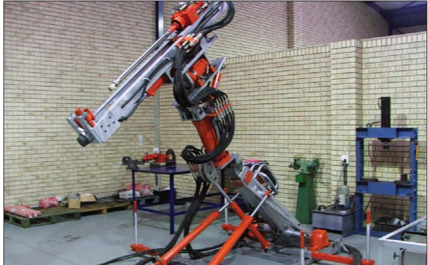
The hot dip galvanized prototype rock drilling machine as supplied.
